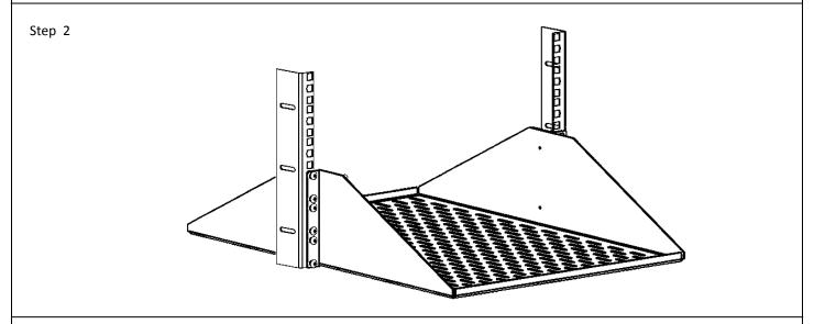
\*\*For the best results install a rack screw in every mounting hole of the rack shelf.\*\*
