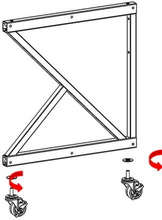
Step 2: Thread each caster all the way in to the insert so that no threads are exposed.
