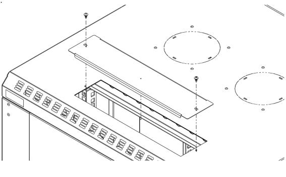
**Step 2:**Reusing the old Phillips head screws, install the brush cover panel as shown.
