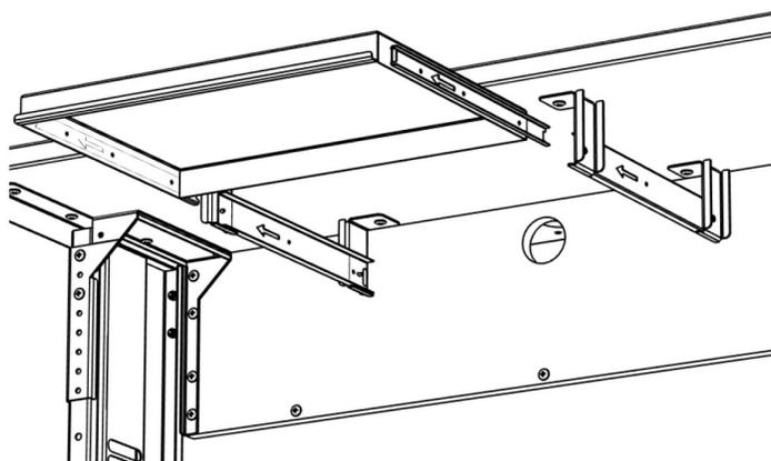
Insert keyboard tray into mounted slides.
