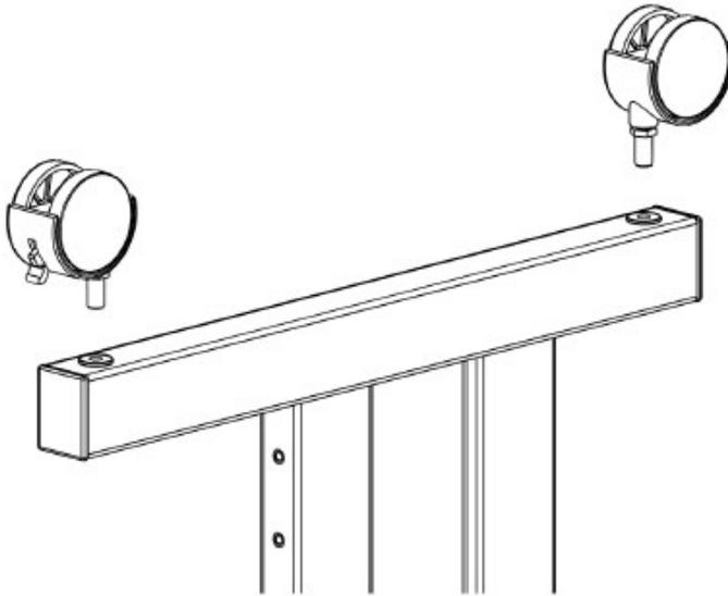
Twist caster into threaded inserts located on the bottom of the training table leg kit.
